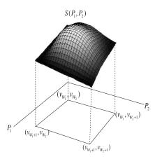
Fig. 2. One of the cases of  $S(p_1, p_2)$  in a subset. It is clear that the minimum value of  $S(p_1, p_2)$  occurs at  $p_1 = v_{w_1}$  or  $v_{w_1+1}$ , and  $p_2 = v_{w_2}$  or  $v_{w_2+1}$  when p is in the subset.
